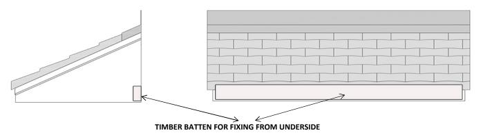
Mark out and pre-drill holes at approx 200mm centres along the canopy fixing flange (upstand).
